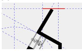
1. Bring the editor functions for the wall back onto the screen. Select any random wall and select the editor functions. The tool bar appears on the screen.
