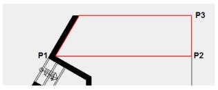
3. You must now specify a height for 3 points of the plane. Click on the corner at **P1**, in the input line enter the height **160** and confirm the value.
