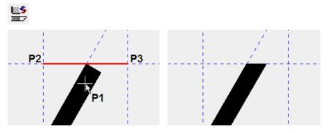
3. Draw the new wall end. The line does not have to start on the outer side of the wall but can overlap if necessary.Start point P2End point double-click P3
