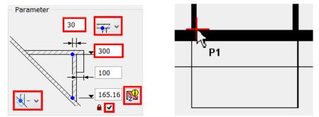
Enter the height of the ridge of the dormer (**300**) and the wall thickness (**30**).
