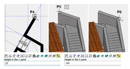
5. The second and third height marker can be selected directly in the 3D model. Rotate in 3D and into the solid display.
