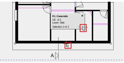
4. Click again on the contour. The cursor changes to a double arrow. This indicates that the cursor is located on a gripper.
