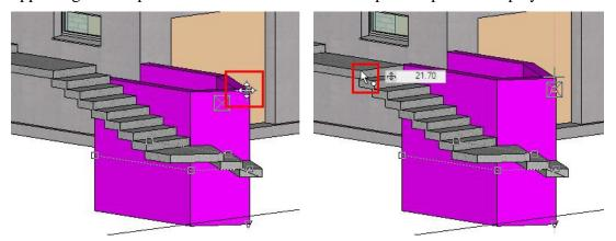
7. On the properties bar the new height is displayed as 261.7. The retaining wall should extend slightly beyond the podium. Change the height to **264**.
