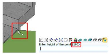
The "transferred" height is written in the input line. In this case this height is directly the desired value. Confirm the value without writing anything into the input line.
