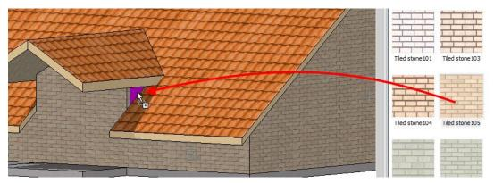
5. Use the centre mouse button to turn the model in such a way that the other dormer side wall is visible and apply the texture to this as well.
