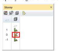
6. The columns must be copied to the ground floor. Use the function COPY TO CURRENT STOREY.
