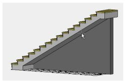
The wall can only have one slope. If there are multiple kinks, the wall must be interrupted.
