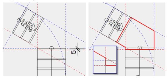
2. Select the function CREATE SLAB and add the values to the properties bar.
