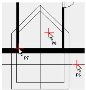
8. Select a placement point. This can be the middle of the dormer or one of the two inner corners (such as P7). It is easiest to set this dormer over a corner. Click on the point **P7**.
