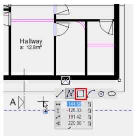
7. Drag the rectangle from point **P1** to **P2**. For point **P2** you require the reference point **RP**.
