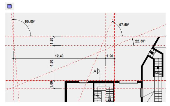
3. Start with the two horizontal planes.Plane 1: Height 0 Colour 313Plane 2: Height 160 Colour 8
