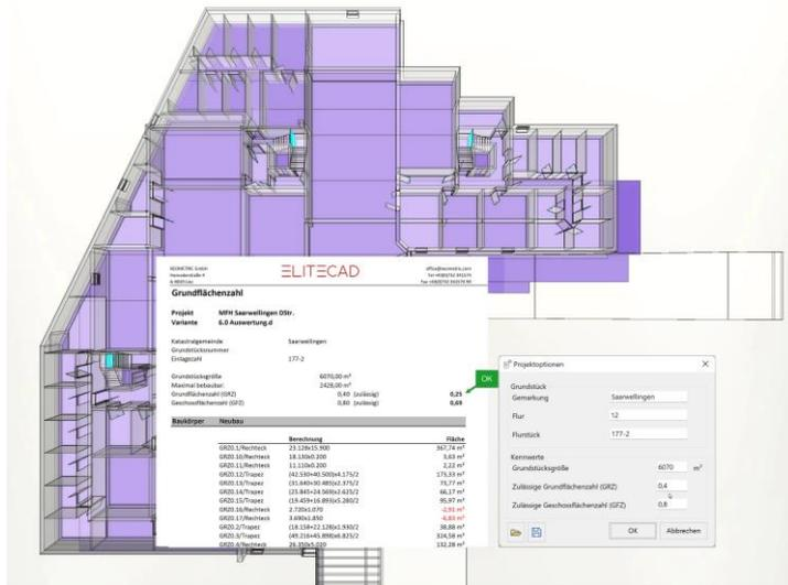
Depending on the project and storey options, ELITECAD Architecture 16 automatically calculates developed areas such as the building coverage ratio (BCR) and floor area ratio (FAR). You can easily select these in the quantity manager and check the associated total and individual areas and rules graphically.
