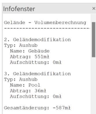
be listed in detail. The information window shows the amount of soil removed and applied for each modification. So that the individual work steps can be distinguished, the log also contains the new names of the respective modifications. Adding everything together provides a sum of the total additions and total removal, which are also output separately and the difference between them is displayed in the property bar as before.
