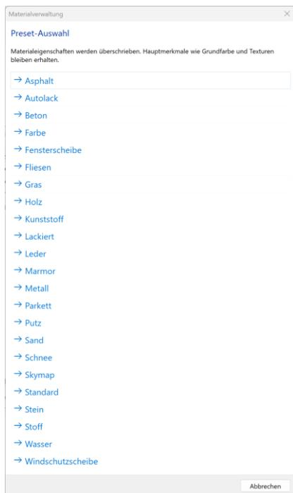
More than twenty fully preconfigured presets and hundreds of multilingual synonyms for the automated parameterisation of materials enable the automatic adjustment of gloss or specularly, for example. Therefore, materials and textures no longer have to be manually configured. All material properties can be preset with one click.
