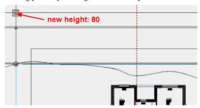
7. In the properties bar, enter the height **80** for the z coordinate and then cancel the function with [Esc].
