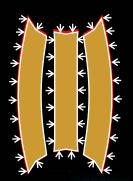
The powerful Material Compensation tool allows MPanel to pre-shrink a panel to account for any post-production stretch in the material. Options allow for any material type and direction.
