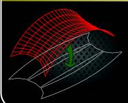
Once the desired 3D shape is achieved, a **single click** creates the flat 2D panels needed to manufacture the design. Choose to create panels in any size, shape or direction. Indicate a specific width and the software will hold the patterns to that dimension. MPanel's reporting tool alerts the user for potential
