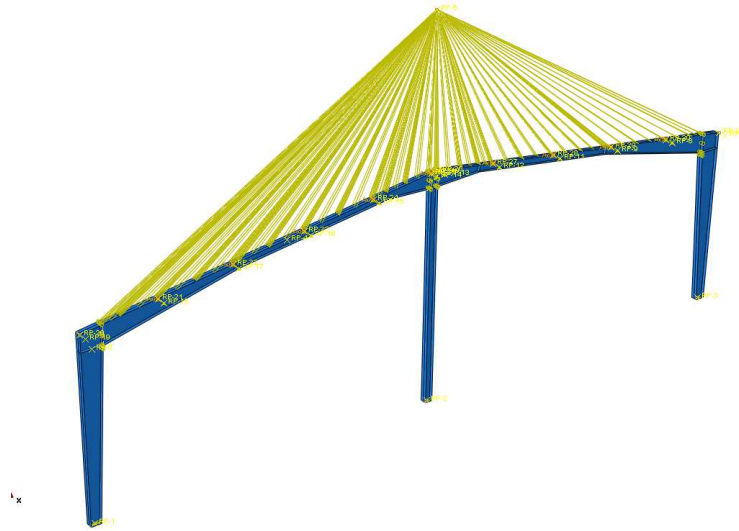
Figure 20: FE model for 2D frame with fixed lateral supports
