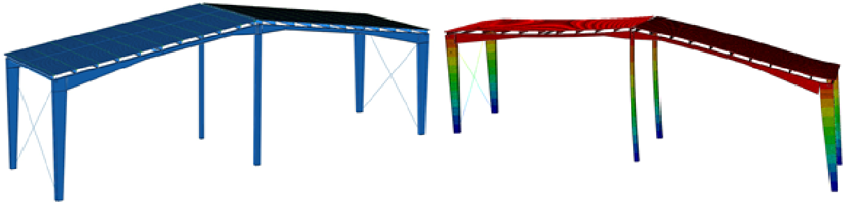
Figure 22: Complex frame and roof model and preliminary sway buckling computed in Abaqus
