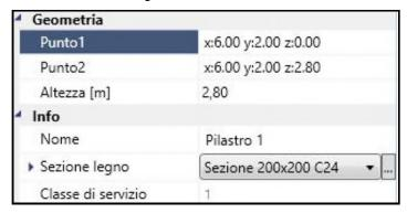
In the box **Geometry** the user can modify the position and the height of the selected Column. In the dialog box **Info** the user can modify the cross-section area. The following informations are reported:
