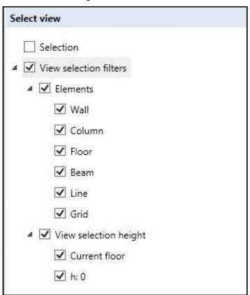
If the user select *Current floor* it will appear a cursor (on the lower right side of the console) which allows to choose the level to display.
