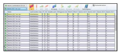
If the user selects the Seismic Combinations (first drop-down menu) he could select one of the 32 combinations to display the results data. The combinations are obtained by changing the centre of mass, to consider the accidental eccentricity, and by changing the values and the directions of the seismic actions (the 100% of the value in one direction corresponds to the 30 % of the value in the other direction.
