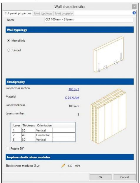
The command *Create CLT wall* allows the user to create a new wall type, defining the geometrical and mechanical characteristics of the CLT panels. In the first window the user has to:
