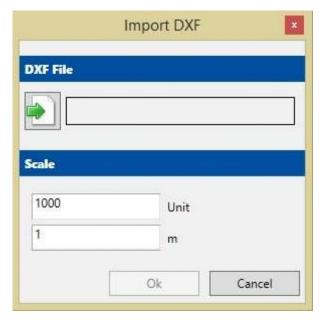
The command is linked to a window in which the user can select the dfx file and specify the importing scale. If the scale is too much small, the software will alert the user.
